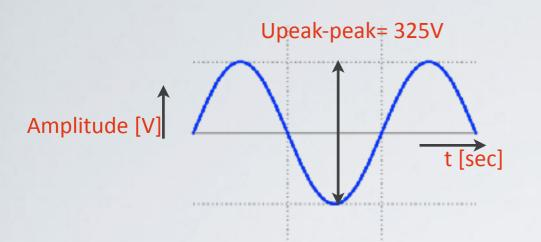
The mains connection on the wall provides us with 230V~ AC /50Hz.
