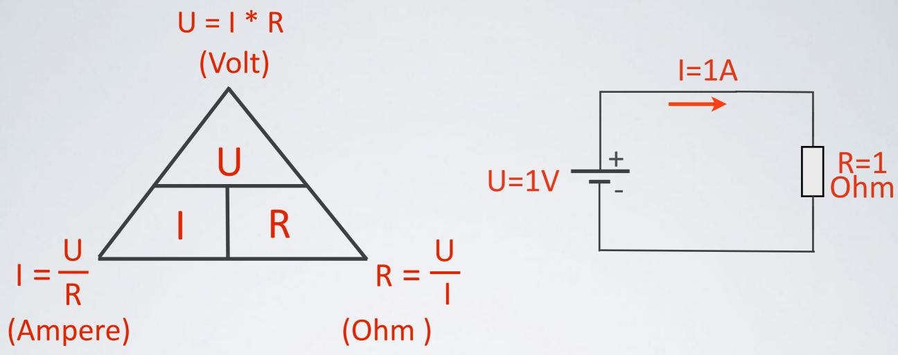
A source of 1 Volt [V] and a resistor of 1 Ohm, will result in a current of 1 Ampere [A]
