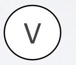
Voltage measurement **R in = very high** Always connect parallel
