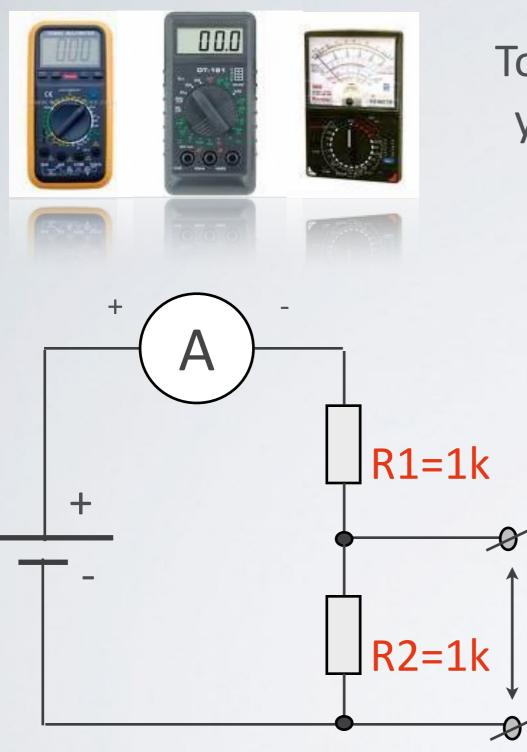
To measure the current with a multimeter, you have to connect the meter in SERIES with the wire. This means you have to disconnect the wire and place the multimeter in BETWEEN...
