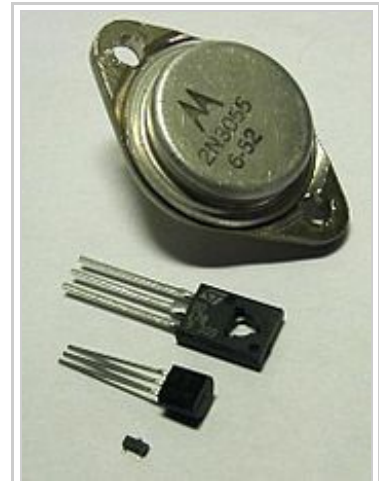
Assorted discrete transistors. Packages in order from top to bottom: TO-3, TO-126, TO-92, SOT-23.
