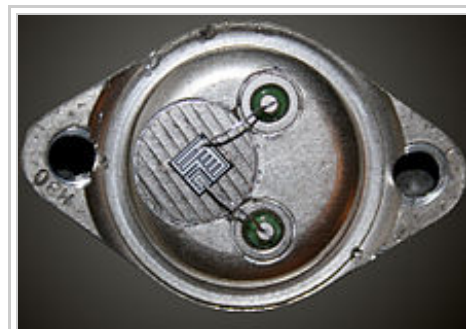
A Darlington transistor opened up so the actual transistor chip (the small square) can be seen inside. A Darlington transistor is effectively two transistors on the same chip. One transistor is much larger than the other, but both are large in comparison to transistors in large-scale integration because this particular example is intended for power applications.
