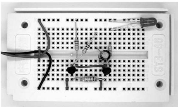
Fig. 35: The LED flasher (F\_Blinker2.jpg)
