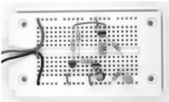
Fig. 37: LED flashing light (Aufbau13.jpg)
