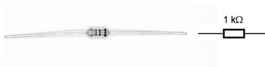
Fig. 6: A resistor (B\_Widerstand.gif)
