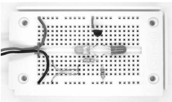
Fig. 15: Examining the current gain of the BC557 (Aufbau2.jpg)
