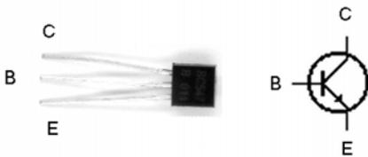
Fig. 7: The NPN transistor BC547 (B\_NPN.jpg)
