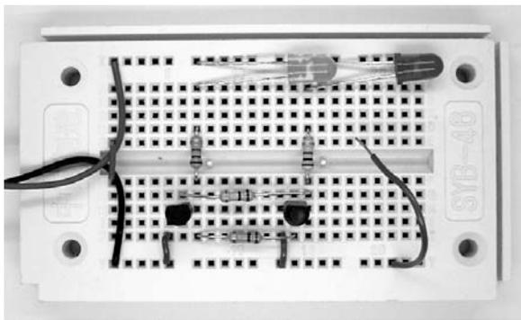
Fig. 29: The flip-flop (F\_Flipflop1.jpg)
