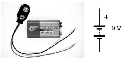
Fig. 3: The battery as it really looks and as schematic symbol (B\_Batterie.gif)
