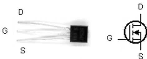
Fig. 9: The MOSFET transistor BS170 (B\_FET.jpg)
