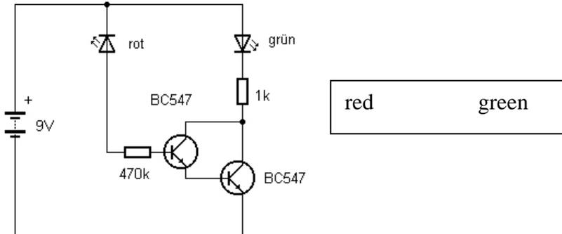
Fig. 22: Gain of the LED reverse current (Schaltung6.jpg)
