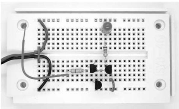
Fig. 21: Sensor amplifier for electric fields (Aufbau5.jpg)
