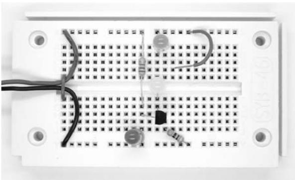
Fig. 25: Stabilisation of LED brightness (Aufbau7.jpg)
