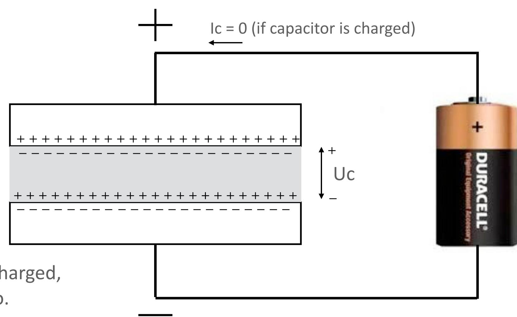
For DC voltage, the Capacitor is a blockade (very high resistor) - the current is zero
