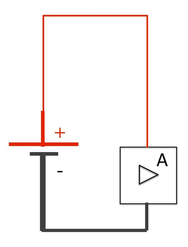
When you connect power to a circuit, use thicker wire for the ground. The ground should always be very LOW IMPEDANT. This means, the resistance should be low. Thicker wire does the job ...
