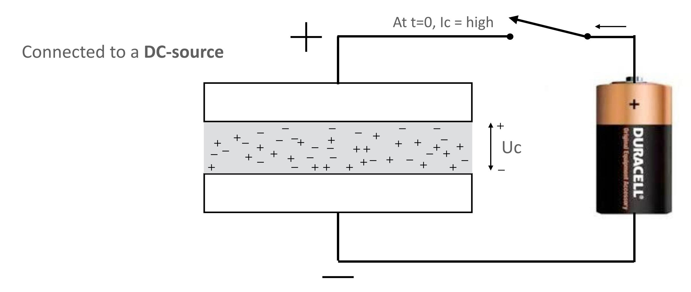
The capacitor will charge until Uc = U battery
