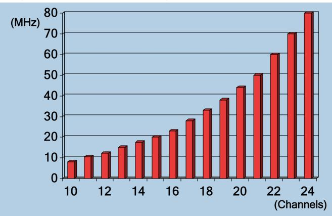
The bandwidth required increases disproportionately with the number of channels. The number of possible IM products runs into thousands. More than 16 channels within the switching bandwidth (24 MHz – 36 MHz) are rarely advisable.
