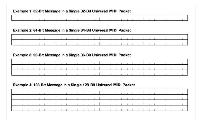
The Universal MIDI Packet format is suited to sending MIDI data over high speed transports such as USB or a network connection or between applications running inside a personal computer OS.
