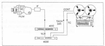
In this instance, the FOSTEX 4010 and 8720 Interface are used to convert the bi-phase signals from a film camera or projector to time code, enabling the synchronous operation of an external audio recorder. The 8720 decodes the bi-phase signal into separate direction and clock signals, which the 4010 uses to generate an appropriate time code. In this manner, live audio may be recorded to the three-track whilst shooting the film, and then subsequently reassembled with the image in the studio.
