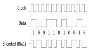
The clear advantage in Biphase Modulation is that the absolute bit rate is irrelevant, as long as it is fairly constant; the time code reader only has to compare the relative lengths of the high and low states in order to clearly distinguish between 0 and 1 at any playback speed.
