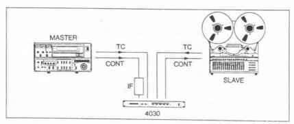
Major differences often exist between tape transports, with respect to the electrical and mechanical characteristics of their external control ports. An interface unit is required to adapt these units to the 4030's own protocol, a process that may involve matching of voltages and impedances, adjustments of timing and logic considerations, and compilation of control signals not directly supplied by the transport.
