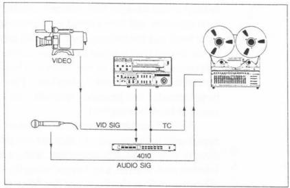
Here, the 4010 is used to generate a time code synchronous with the video signal from a camera. This time code is simultaneously recorded on the video and audio recorders' cue tracks, along with the live picture and sound programmes. The audio and video portions may be later synchronized for editing and playback thanks to this time code, via the 4030 Synchronizer.
